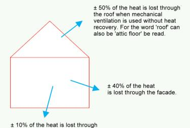
If insulation is applied, only the outer shell must be insulated. This is usually the roof, the floor/facade that borders the outside air/crawl space or the ground).
